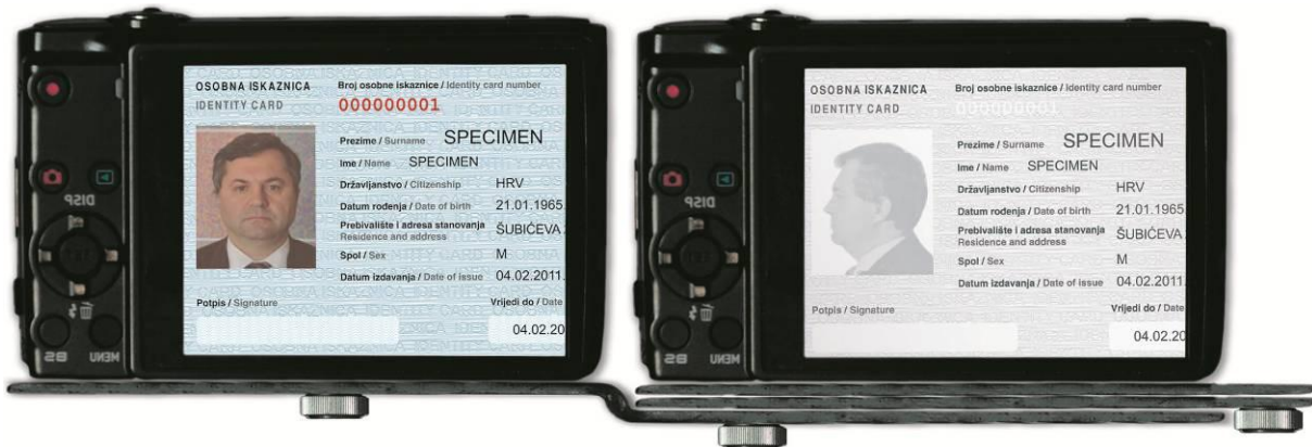
Picture 2. ZRGB cameras with a portrait image: the visual and near infrared specter (2)
